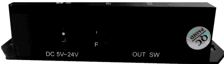
Left pannel : DC power supply, LED: I/P SW : Force output resolution
