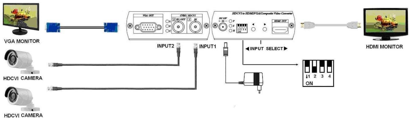
\* Allow two camera inputs with 2 outputs: HDMI, VGA as a switcher.
