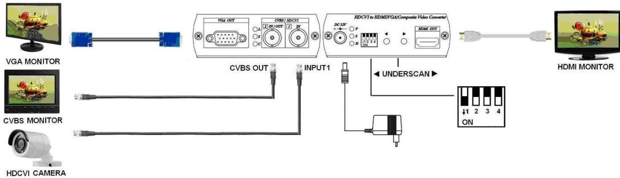
\* 3 outputs: HDMI, VGA, CVBS could be display simultaneously.
