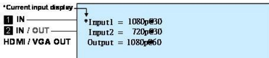
Button as input selection, press ◀ to display Input 1 picture, press ▶ to display input 2 picture, the current input display will be add 「\*」 symbol marked.
