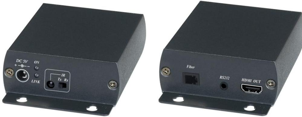
HE01F is an Optical HDMI Extender that overcomes the length restriction of standard HDMI cables by using optical fiber to send high definition audio and video signals over large distances. It also built in RS232 and IR to extend the IR remote control and transfer RS-232 (up to 115kbps) in both directions, allows you to connect serial devices such as touch screens and barcode scanners.
