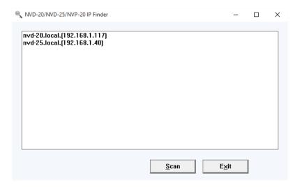
When the utility scans the LAN that the computer is connected to, it displays the current IP address for any NVD-25 units found on this local IP network. Double clicking on the device listed will automatically open your computer's default web browser and navigate to the login page of the NVD-25.
