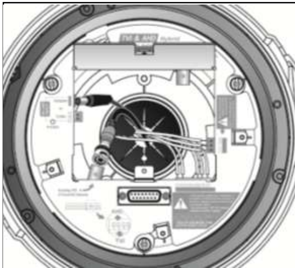
④ Open housing connecting cover and connect Power, data, video cables
