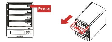
**Step 4** Mount your hard drives onto the removable drive tray and secure it with the screws included in the accessory kit to avoid any damage to the hard drive due to accidental movements.
