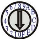
HE05BT and HE5BER I must setting at same channel in order to do mutual transmission. Rotary switch to be follow 16 HEX, could switch " 0 ~ F " total 16 channels, A = channel 10, B = channel 11, others channel same as 16 hex conversion. HE05BT host channel setting must setup as the only one channel to avoid conflict with any other HE05BT transmitter.
