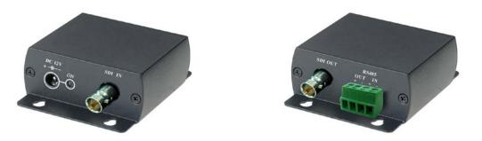
SR02 is a repeater for HD-SDI links operating with  $75\Omega$  coax cable. It can be daisy chained together up to 5 pieces of SR02 with working distance 1KM. When using multiple SR02 repeaters installation, the repeater power could be send over coax cable from the remote repeater (nearest the DVR). It also support RS485 data control as well. The application could be using for HD CCTV HD-SDI camera extra long range video monitoring.
