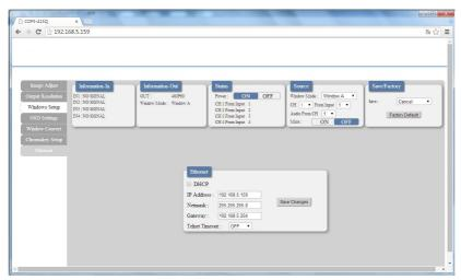
Clicking on the 'Ethernet' tab to reset the IP configuration. The system will ask for a reboot of the device every time when any of the settings is changed. The IP address needed to access the Web GUI control will also need to be changed accordingly on the web address entry bar.
