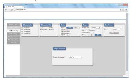
Clicking on the 'Output Resolution' tab to set the output display resolution.
