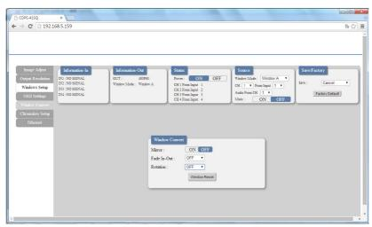
Clicking on the 'Window Convert' tab to set the output display angle. **Note: This function is only available under window A~D.**
