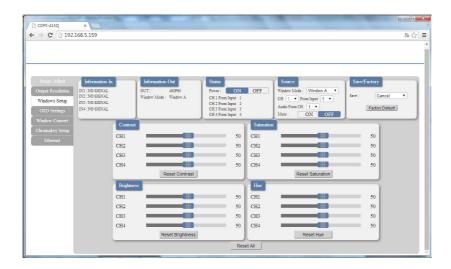
Click on the 'mage Adjust' tab to control power, Window Mode and the window setting.
