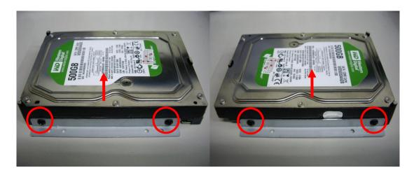
Step 2) Place the HDD on the HDD plate and screw it as indicated.
