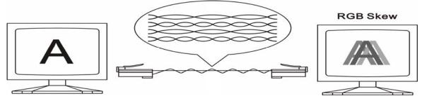
2. Recommend to use following cabling way to reduce skew status, to add special made "skew immunized adaptor", 2 pieces included at the package. Total distance
