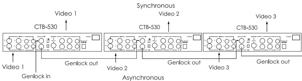
**75 ohm load switch :** When CTB-530 Genlock out is not connected to the Genlock in of another unit, set the switch to ON. Set to OFF if it is connected to another unit.
