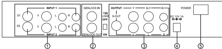
Genlock out is a loop-through of Genlock input which made possible the synchronization between multiple video sources by connecting Genlock out to the Genlock in of the next unit, and repeat it.
