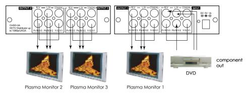
2. Works as a 1-in 3-out distribution amplifier for HD RGBHV video source.
