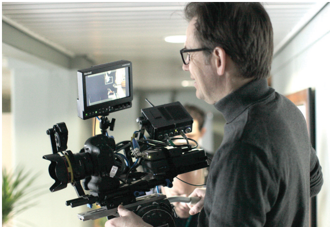
The EOS 1D Mark IV with Scorpio remote, Marshall monitor, Red Rock baseplate, Globalmediapro battery and Blackmagic Design converter. Below: DoP Pål Bugge Haagenrud with the Canon rig
